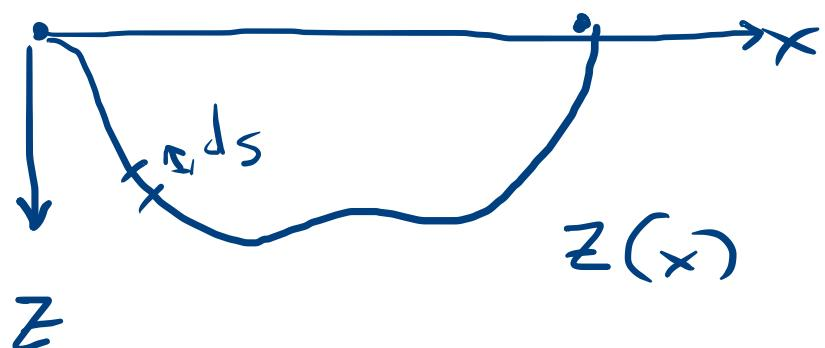
$$T_{A \rightarrow B} = \int_A^B dt = \int_A^B \frac{ds}{v}$$
