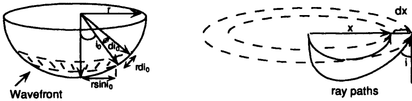
FIGURE 3.6 The area, which is inversely proportional to energy, for an expanding spherical wavefront.
