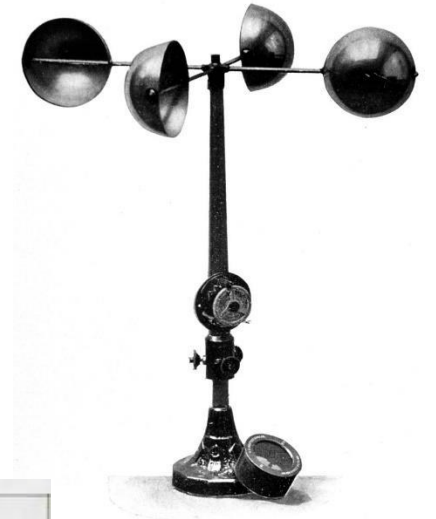
THE ROBINSON ANEMOMETER.
