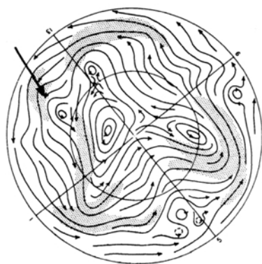
Figure 32. Streak photographs of the upper surface of the dishpan in an experiment revealing chaotic behavior, accompanied by streamline analyses based on the photographs. The right-hand patterns follow those on the left by one rotation. Photographs and analyses by Dave Fultz, reproduced by permission of the American Meteorological Society.
