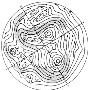
Figure 32. Streak photographs of the upper surface of the dishpan in an experiment revealing chaotic behavior, accompanied by streamline analyses based on the photographs. The right-hand patterns follow those on the left by one rotation. Photographs and analyses by Dave Fultz, reproduced by permission of the American Meteorological Society.
