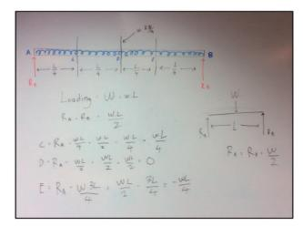
FIG. 4. Shearing force diagram for uniformly distributed load. This figure appears in colour in the online version of *Teaching Mathematics and its Applications*.
