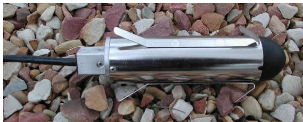
Figure 12: An IMS tri-axial 4.5 Hz borehole geophone. The sensor is usually installed in 10 m holes of diameter at least 76 mm. The signals from such sensors are less noisy and have less distortion than signals from surface-mounted seismic sensors.
