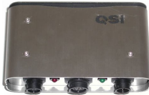
Figure 14: The GSi seismic data acquisition unit from ISS International. This unit is a full seismic station that uses less than 0.11 W of power and has been certified for use in explosive gas environments. The unit is very compact (130 mm × 80 mm × 30 mm) and records digital seismograms from a tri-axial geophone at a sampling rate of 5000 Hz.
