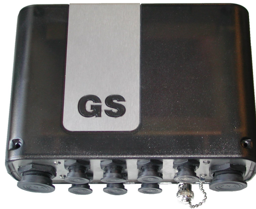
Figure 13: The GS seismic data acquisition unit from ISS International. With a frequency bandwidth of 0.3 - 48000 Hz and a dynamic range of 129 dB at 6000 Hz sampling rate, this seismic station meets the requirements of the typical seismic monitoring system. The unit is compact (140 mm × 200 mm × 65 mm) and has a power consumption of 3 W. Digital seismogram data is transmitted to the central site and can also be stored locally on a USB disk.
