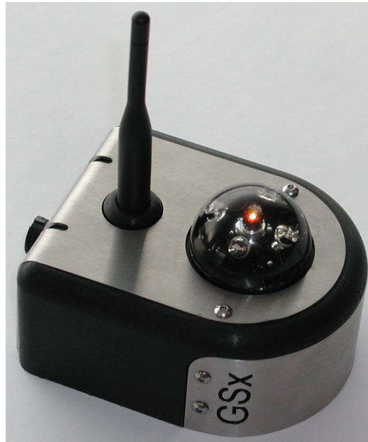
Figure 15: The wireless GSx seismic data acquisition unit from ISS International. This unit monitors an internal 14 Hz uni-axial geophone and reports the micro-seismic activity rate to the closest GS each minute. The device is powered from a rechargeable internal battery and communicates via a spread-spectrum digital radio, using other GSx units as relays if necessary. The device has bright lights that can be turned on remotely to warn local users of unusual micro-seismic activity rates.
