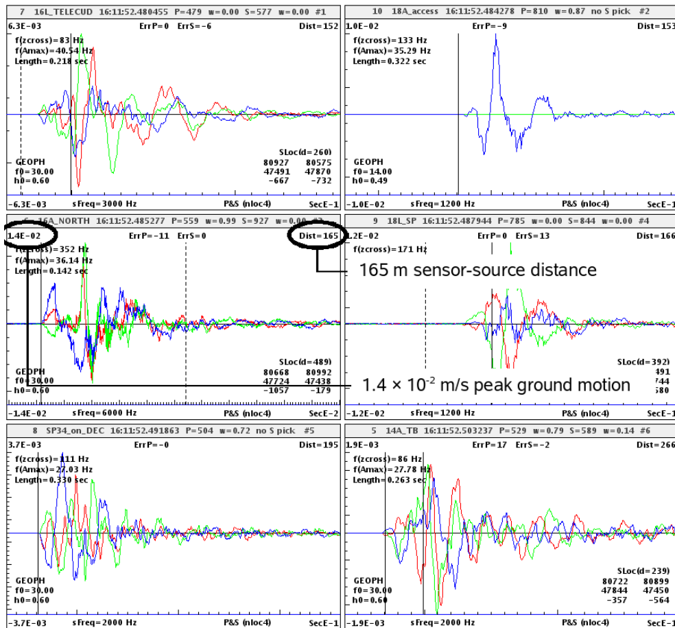
Figure 11: Seismograms recorded by an array of 14 Hz and 30 Hz borehole geophones for a magnitude +1.8 event.
