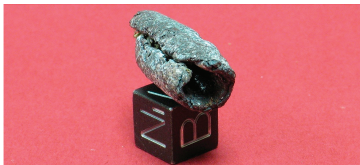
FIGURE 2 Meteoritic metal bead formed from the Anoka (Minnesota) iron using wood-fueled fire for heating and lithics for deformation (i.e. hammered using rocks). PHOTO: SMITHSONIAN INSTITUTION
