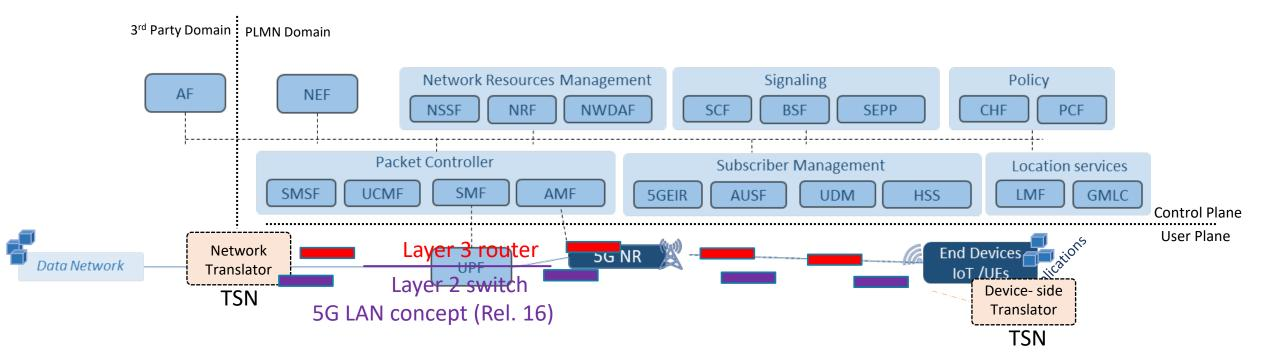
For a UE the PDU session is supported by ONE CN tunnel and ONE OR MORE AN tunnels (DRB)
