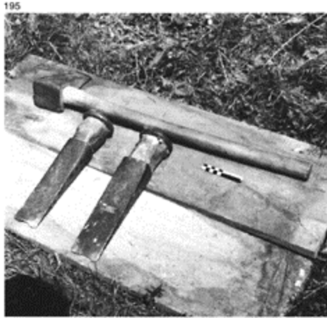
195 Splitting axe or cleaver and wedges, Vosges Mountains, twentieth century.
