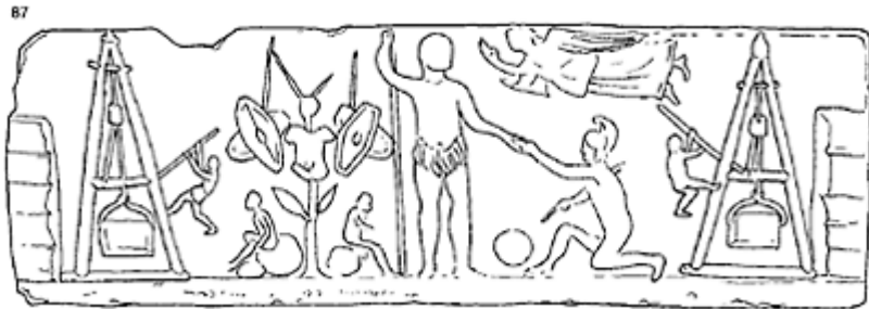
87 A representation of two winch cranes operated by levers; the stones are held by grips. Terracotta relief
