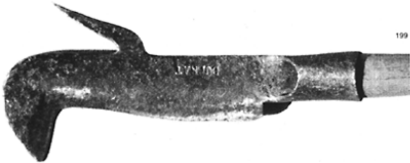
199 Modern billhook. Total length including handle: 1.5m; length of blade: 30cm.
