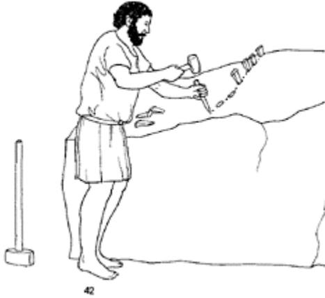
42 Drawing showing splitting a block using wedges.
