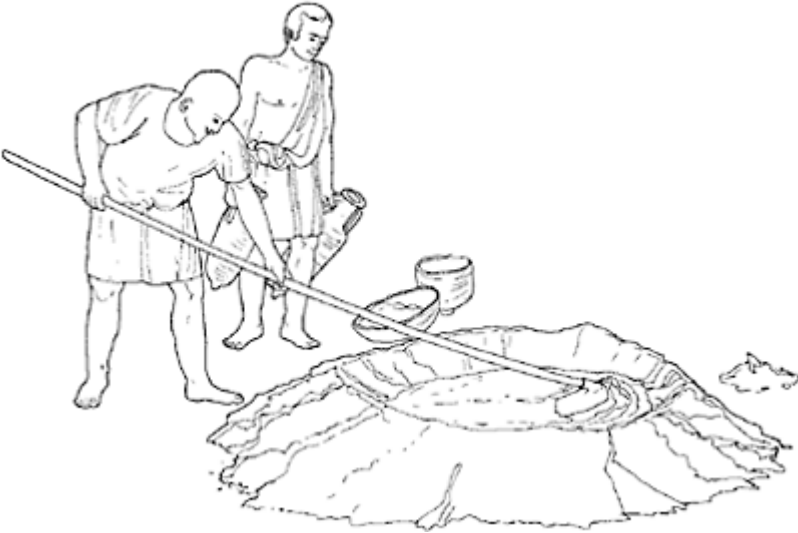
163 Preparation of lime mortar or tempering; mixing sand, fat lime and water using a hoe.
