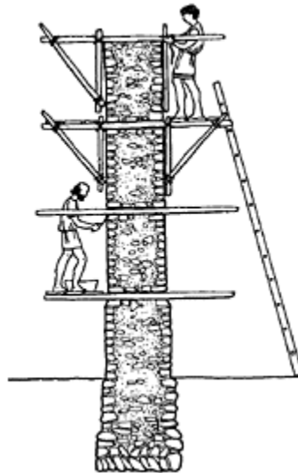
183 Socketed Scaffolding with transverse putlogs.
