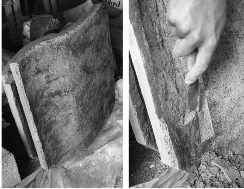
Figure 20. After drying, the replica tile is stiff enough to remove from the base mold and stand on end ( left ); the clay is resistant but can be trimmed by peeling off layers with a metal spatula ( right ). Photos A. Trdan
