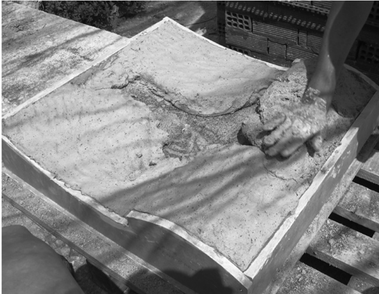
Figure 17. Packing clay slabs into the base mold to form a replica tile. Photo A. Trdan
