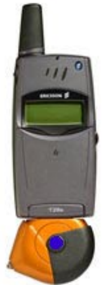
„BarMailer“, a snap-in bar code reader for mobile phones
