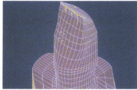
Fig 2 3-D FEA model. The four arrows in the center of the palatal surface indicate an area of oblique stress induction.
