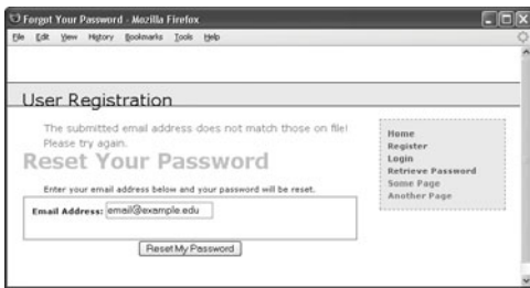
Figure 16.28 If the user entered an email address that is not found in the database, an error message is shown.
