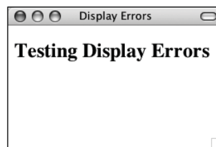
Figure 7.11 With display_errors turned off (for this page), the same errors (Script 7.1 and Figure 7.10) are no longer reported. Unfortunately, they still exist.
