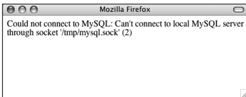
Figure 8.5 Another reason why PHP might not be able to connect to MySQL (besides using invalid username/password/hostname/database information) is if MySQL isn't currently running.
