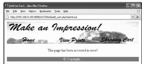
Figure 17.36 The add_cart.php page will only add an item to the shopping cart if the page received a valid print ID in the URL.
