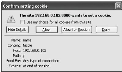
Figure 11.6 If the browser is set to ask for permission when receiving cookies, you'll see a message like this when a site attempts to send one (this is Firefox's version of the prompt).
