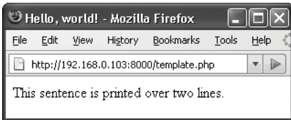
Figure 1.8 The return in the HTML source (Figure 1.7) has no effect on the rendered result. The only way to alter the spacing of a displayed Web page is to use HTML tags (like <br /> and <p> ).
