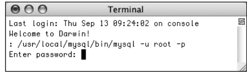
Figure 4.4 Access the mysql client by entering the full path to the utility, along with the proper arguments.
