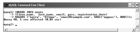
Figure 5.7 This query inserts a single record into the users table. The 1 row affected message indicates the success of the insertion.
