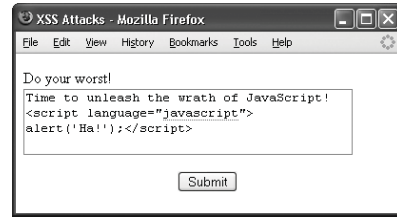
Figure 12.11 The malicious and savvy user can enter HTML, CSS, and JavaScript into text inputs.
