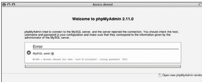
Figure 4.9 Every client application requires a proper username/password/hostname combination in order to interact with the MySQL server.
