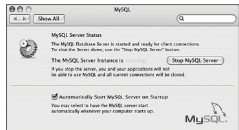
Figure A.10 The MySQL preferences pane can be used to control the MySQL database server.
