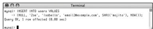
Figure 5.8 Another record is inserted into the table, this time by providing a value for every column in the table.
