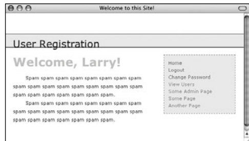
Figure 16.26 Upon successfully logging in, the user will be redirected to the home page, where they will be greeted by name.
