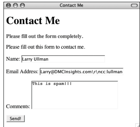
Figure 12.4 The email was not sent because of the very bad characters used in the email address.
