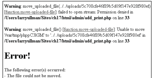
Figure 17.10 If the uploads directory is not writable by PHP, you’ll see errors like these.
