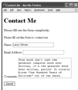
Figure 10.2 The contact form will remember the user-supplied values in case it is not completely filled out.
