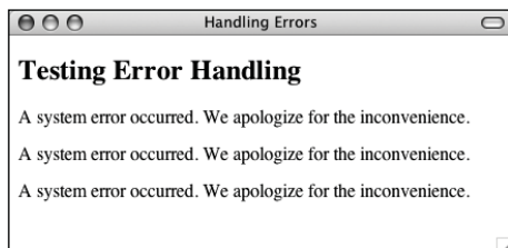
Figure 7.17 Once a site has gone live, more user-friendly (and less revealing) errors are printed. Here, one message is printed for each of the three errors in the script.
