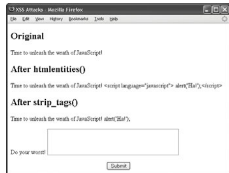
Figure 12.13 Thanks to the htmlspecialchars() and strip_tags() functions, malicious code entered into the a form field (see Figure 12.11) can be rendered inert.
