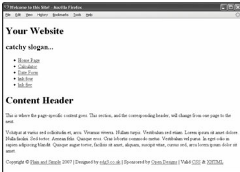
Figure 3.6 This is the same HTML page without using the corresponding CSS file (compare with Figure 3.4).
