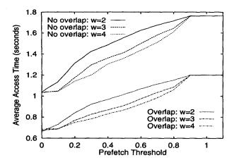
Figure 5: The average file access time versus the prefetch threshold, p. The upper set of curves are for the no-overlap model described in Section 4.2 while the lower set is for the overlap model. Within each set, the lookahead window size, w, is also varied.
