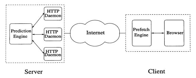
Figure 2: This figure depicts the architecture of the system with prefetching. On the server side, the set of httpd processes (one per active client) communicate with the prediction engine, which makes prefetching-related predictions. On the client side, the prefetch engine initiates prefetching based on advice from the server and some other factors. The bidirectional arrows denote local communication between entities at the server and at the client.
