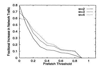
Figure 6: The fractional increase in network traffic versus the prefetch threshold, for different values of the lookahead window size, w. The curves shown are for the overlap model; those for the no-overlap model are essentially the same.
