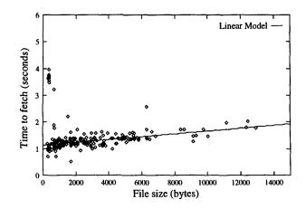
Figure 4: A scatter plot of the time taken by a client at UC Berkeley to fetch files (Web pages, inline images, etc.) of different sizes from Digital's Web server, and the line corresponding to the linear regression model.
