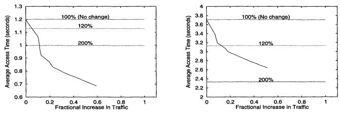
Figure 8: The average file access time with and without prefetching, both with UC Berkeley-Digital network model (figure 8) and a 28.8 Kbps modem link (figure 9). The solid curve in each figure corresponds to the case of prefetching with a lookahead window size of 4. The horizontal, dotted lines correspond to non-prefetching systems with available bandwidths of 100%, 120%, and 200% of that used when simulating the prefetching system.
