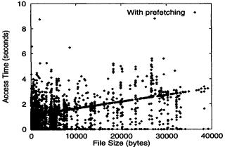
Figure 13: A scatter plot of access time versus file size with the prefetch threshold set to 0.4 and the lookahead window size set to 4.
