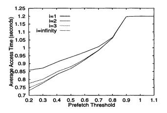
Figure 10: The average file access time versus the prefetch threshold, p, for different values of i.
