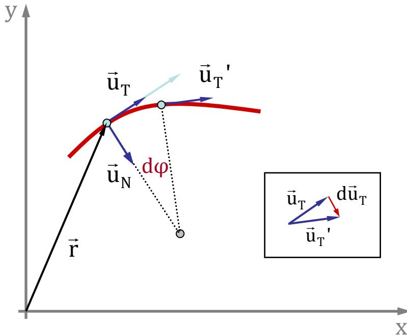
$$\vec{a} = \frac{d\vec{v}}{dt} \Rightarrow \vec{a} = \frac{d}{dt}(\vec{u}_T v) = \vec{u}_T \frac{dv}{dt} + \frac{d\vec{u}_T}{dt} v$$
