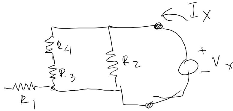
$$-\frac{V_x}{I_x} = R_2 \parallel (R_4 + R_3)$$
