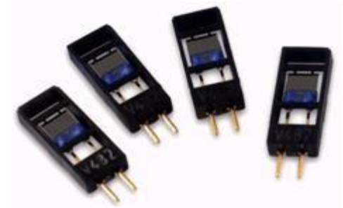
\Delta C \propto \text{humidity} humicap
