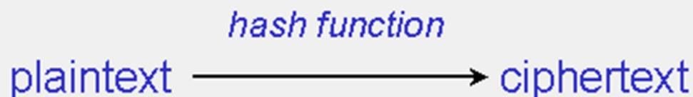
**C) Hash function (one-way cryptography). Hash functions have no key since the plaintext is not recoverable from the ciphertext.**
