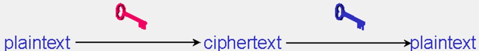
**B) Public key (asymmetric) cryptography. PKC uses two keys, one for encryption and the other for decryption.**
