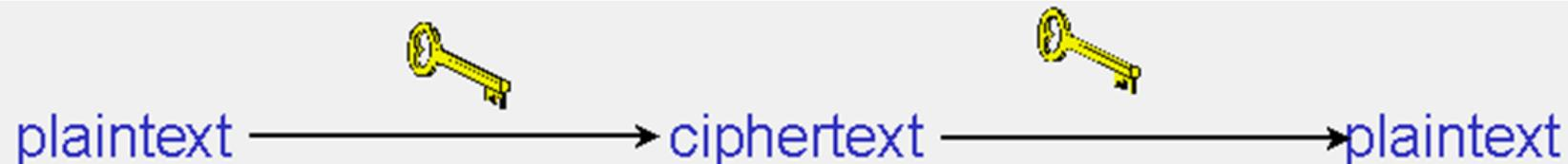
**A) Secret key (symmetric) cryptography. SKC uses a single key for both encryption and decryption.**
