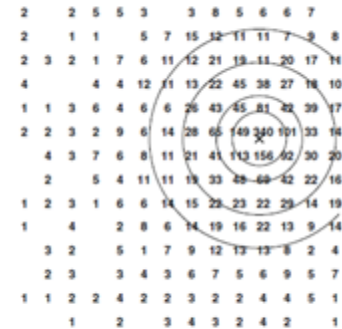
Fig. 8.13. Map of an air shower in a 196 detector array on a 15 m grid. The densities from (8.18) fluctuate with a Gaussian distribution with \sigma = \sqrt{\rho} . Because of that some detectors do not trigger.
