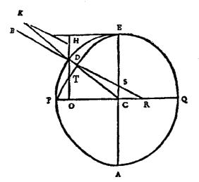
also what was explained by it, but, making the shape of the Earth a little diminished and flattened toward the poles such that the axis PQ would be shorter than the diameter EA. Let BDSR be drawn parallel to KH, cutting EA and PQ at S and R. The thread KH, which supports the lead weight, or rather its parallel BD, must meet the surface of the ocean at right angles. This thread hangs such that KD is to
