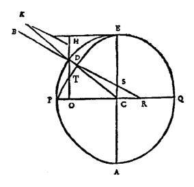
In order to find next what the curved line EDP is, I imagine the canal ECD full of water, and drawing DO perpendicular to the axis PC, I take CO to be x, and OD to be y, the other lines being named as before. It is certain that the water from EC and that from DC must again be counterbalanced. And likewise, this must happen regardless of how we understand the canal to be made, provided that it ends on
