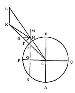
In order to know now what the position of thread KH must be and how much less the lead shot H weighs in this way than if it were to hang perpendicularly (p.148) along KD, it is necessary to consider point H being pulled by three threads, HC, HM and HK. HC pulls it toward the center of the Earth with all the weight that the lead shot would have if the Earth was immobile. But HM pulls it from this direction with the force that the motion of the Earth gives in circle DN. And the
