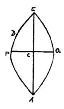
So, if the Earth, with diameter EA of its true length, turned 17 times faster than it does on its axis PQ, (for then the centrifugal force at E would be equal to the gravity toward the center, by the demonstration that is in (p.158) this Discourse), it would have the figure of a body like the two half parabolas opposed, PEC and QEC, turning around its axis PQ. And we see that there is here the greatest centrifugal force that we can suppose; for, if we had made it greater
