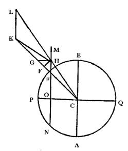
289 to 1 and of EC to DO.<sup>36</sup> But the angle HDK is also known, being equal to that of the latitude of Paris, namely as some 48 degrees 51 minutes. Then we will know the proportion of DK to KH, which is that of the absolute gravity of bodies to that which they have in Paris, and which is likewise the length of the pendulum on the immobile Earth to the length that it must have at this parallel, according to what has already been said. And seeing that the length of a seconds
