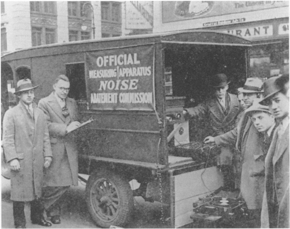
Figure 4. The noise-measuring truck of the Noise Abatement Commission of New York City, circa 1929. The truck was manned by acoustical engineers from Bell Telephone Laboratories and the Johns-Manville Corporation (manufacturers of acoustical building materials) and employees of the New York City Department of Health. It logged over 500 miles on the city's streets, making over 10,000 "observations" at 138 different points in the city. (From Edward F. Brown et al., eds., City Noise [New York: Department of Health, 1930], on page 32.)
