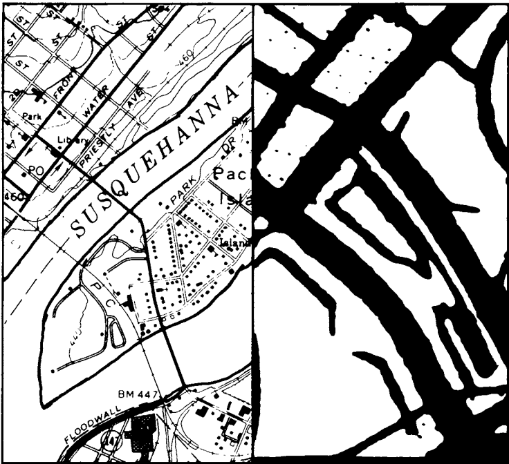
FIGURE 3.4. Area near Northumberland, Pennsylvania, as portrayed on topographic maps at 1:24,000 (left) and 1:250,000, enlarged to roughly 1:24,000 for comparison (right).
