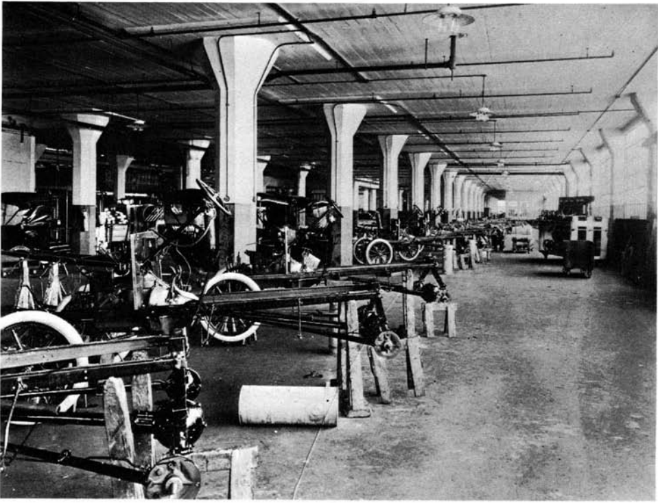
FIGURE 6.14. Static Assembly of Model T Chassis, 1913. Unfortunately, the moving assembly gangs were not included in the photograph. (Henry Ford Museum, The Edison Institute. Neg. No. 0-1267.)
