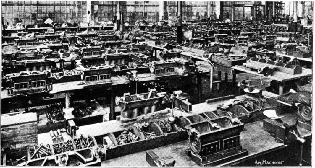
FIGURE 6.11. Engine Assembly, Highland Park, 1913. Individual workmen assembled entire engines by themselves. Unlike most of the photographs used by Fred Colvin in 1913, the original print of engine assembly no longer survives in the Ford Archives. ( American Machinist , June 12, 1913. Eleutherian Mills Historical Library.)
