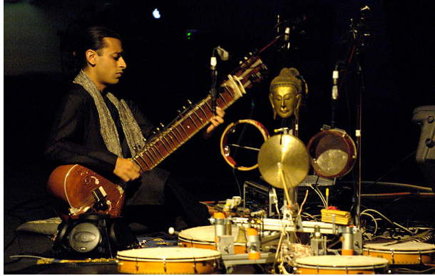
Figure 8. MahaDeviBot communicating in real-time with a performer using sensor on the ESitar and audio analysis
