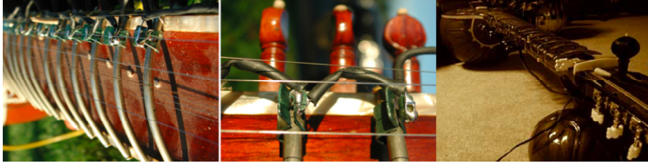
Figure 4. Fret-detection resistor network on the ESitar for capturing left-hand position.
