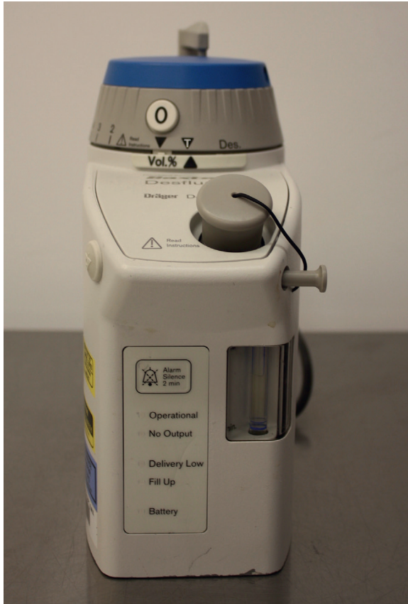
Fig. 16.8 A TEC 6 desflurane vaporiser. Note it is set at the 'T' transport setting for safe transport, and an electrical supply is required to heat the vaporising chamber.
