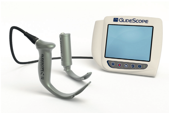
Fig. 23.15 GlideScope videolaryngoscope – Macintosh blades in the background and hyperangulated blade in the foreground. (Reproduced from https://verathon.com/glidescope-titanium-reusable/ . © Verathon Inc.)
