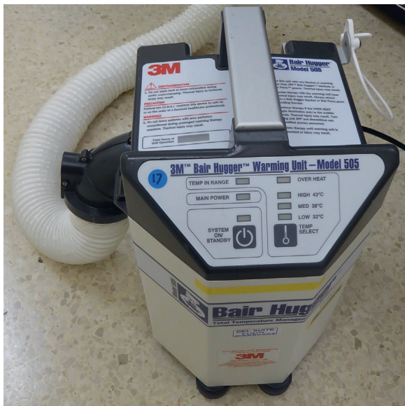
Fig. 16.44 The power unit which generates heated air that is forced through a hose connected to a disposable blanket. (Image copyright 3M.)
