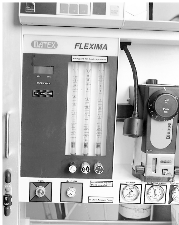
Fig. 16.5 Flowmeters with mechanical linkage between nitrous oxide and oxygen.
