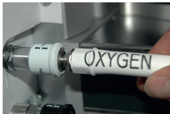
Fig. 23.47 Mini Schroeder valve, a source of high-pressure oxygen on the anaesthetic machine.
