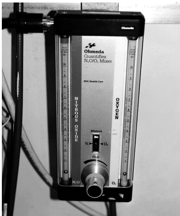
Fig. 16.4 A Quantiflex flowmeter. The required oxygen percentage is selected using the dial, and total flow of the oxygen/nitrous oxide mixture is adjusted using the grey knob.
