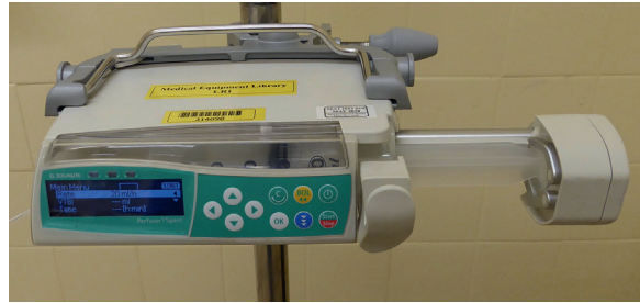
Fig. 16.41 A syringe driver. An electric motor drives a plastic syringe plunger to infuse the contents of a syringe.
