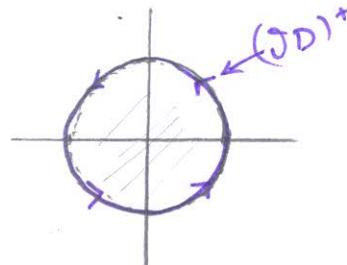
$$(\partial D)^+ \vec{r}(+) = (6wt, npt), \quad t \in [0, 2\pi]$$
