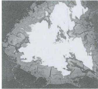
Figure 10.8. Rammelsbergite (white) partly replaced by a Ni-arsenate (grey).
