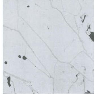
Figure 8.2b. SEM photomicrograph of specular hematite (light grey) with goethite along grain boundaries. Wabush deposit.
