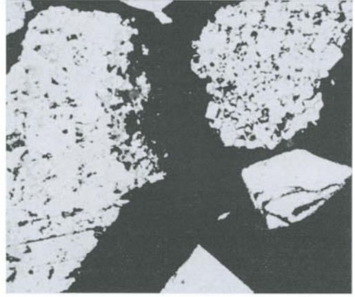
Figure 3.3b. High magnification photomicrograph of two grains of vuggy pyrite (light grey) with minute ( $>1 \mu\text{m}$ ) galena (grey) inclusions in vugs.
