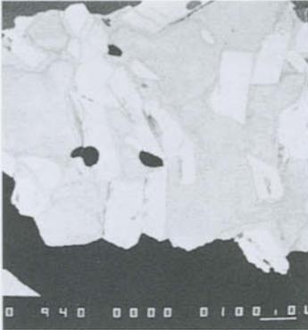
Figure 8.5. SEM photomicrograph of a polished section of hematite (variety specularite) (white) partly replaced by goethite (light grey). Wabush deposit.
