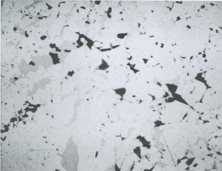
Figure 3.4. Chalcopyrite (grey) in interstices between pyrite grains in massive pyrite (light grey).
