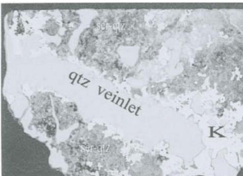
Figure 7.1. Potassic alteration: K-feldspar (K, white) along edges of quartz veinlet, and associated with sericite-quartz (ser-qtz), (modified from Osatenko and Jones, 1976).
