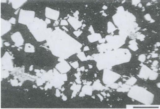
Figure 4.7. Disseminated pyrite + chalcopyrite (DP+C) ore type showing disseminated pyrite (white) and minor chalcopyrite (light grey) in gangue (black). Bar scale = 325  $\mu\text{m}$ .
