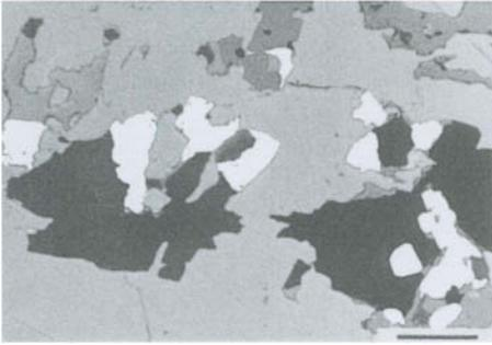
a). Irregular Au-Ag-Hg alloy grains (white) in pyrite (very light grey) associated with galena (grey) freibergite (dark grey) and gangue (black). Bar scale = 40  $\mu\text{m}$ .
