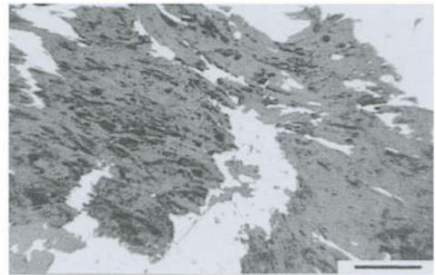
b). Chalcopyrite and minor pyrite and pyrrhotite (white, not differentiated) in chlorite (dark grey). Bar scale = 325  $\mu\text{m}$ .
