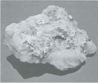
Figure 6.1. Hand specimen of very high grade gold ore. The gold (white) occurs as veinlets in quartz. Timmins, Ontario.
