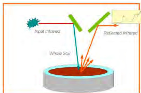
Figure 1. Basis of soil analysis using diffuse reflectance infrared Fourier transform (DRIFT) spectroscopy.
