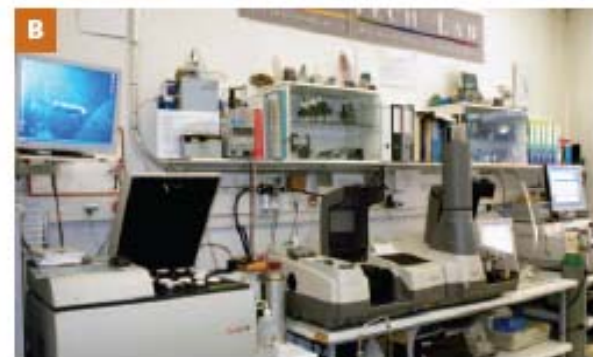
FIGURE 4 In modern gemology laboratories, visual observation is important. At GemTechLab (Geneva), roughly one-half of the room is occupied by binocular microscopes (A), while the other half (B) contains analytical instruments such as ED-XRF, FT-Raman, FTIR, and UV-NIR spectrometers.
