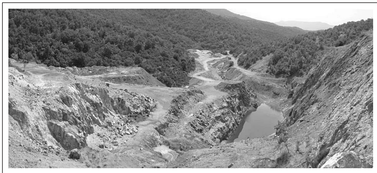
Figure 4. General view of the open pit mine area. Mining waste dumped downstream and waste heap drainage escaping towards the brook.
