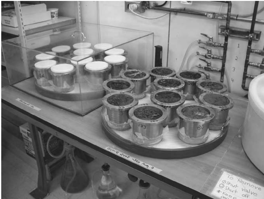
FIGURE 72.2. Example of tension plate apparatus (high-tension system) loaded with 10 cm inside diameter by 11 cm long intact soil cores. The cores are resting on a nylon cloth (15 \mu\text{m} pore size), which overlies a 0.5 cm thick layer of glass bead tension medium (25 \mu\text{m} mean particle diameter), which in turn overlies a 53 cm diameter ceramic disk ( -10 m bubbling pressure) sealed within a PVC backing plate. To minimize biological growth and evaporative water loss, the cores are loosely capped with opaque plastic lids and the entire tension plate is covered with an acrylic lid. The trap (small flask) and overflow reservoir (large flask) for the vacuum system (Figure 72.1b) can be seen below the plates. Tygon tubing (1/4-in. i.d. by 1/8-in. wall) connects the trap to the inflow–outflow port of the tension plate via a hole drilled through the bench top.
