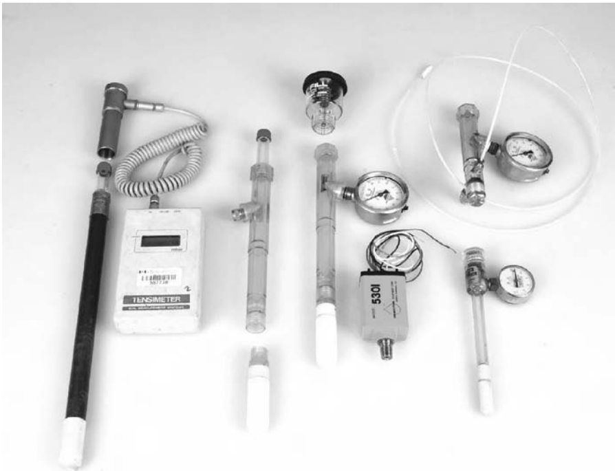
FIGURE 71.2. Some selected tensiometers. From left to right: tensiometer ® fitted with septum cap and tensiometer readout device; customized tensiometer modified to accept a gauge or pressure transducer readout; tensiometer showing two optional screw caps and a manual gauge readout; pressure transducer for use as an alternative to a manual gauge; tensiometer fitted with a flexible “spaghetti” tubing and a mini porous cup; scaled-down tensiometer with midsized cup. Note that all the porous cups are ceramics, which is the most popular and least expensive of the available porous materials.
