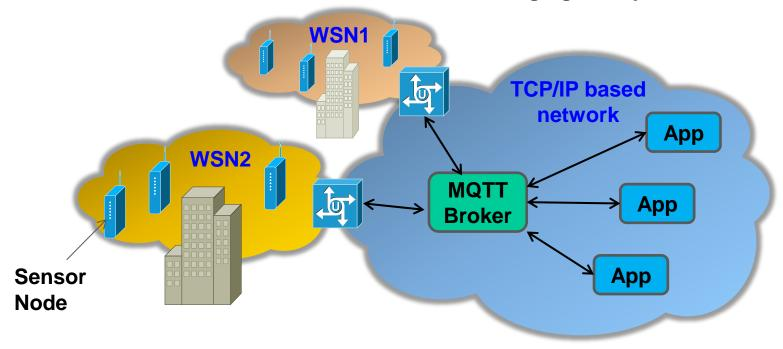
MQTT-S is an extension of MQTT for WSNs.
