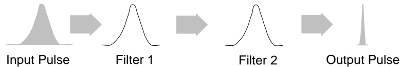
Figure 335. Effect of Multiple Filters on Signal Pulse
