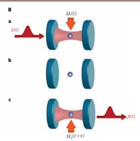
with 1/g, the atomic state is mapped from  $|b\rangle$  to  $|a\rangle$  with the accompanying coherent absorption of one intracavity photon. Conversely, in panel **A**, **b** of the figure, by turning a control field  $\Omega_2(t)$  from off to on, the atomic state is mapped from  $|a\rangle$  to  $|b\rangle$  with the transfer of one photon into the cavity mode.
