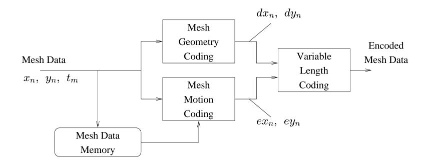
Fig. 12.11: 2D Mesh Object Plane (MOP) Encoding Process
