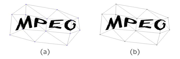
Fig. 12.15: Mesh-based texture mapping for 2D object animation.
