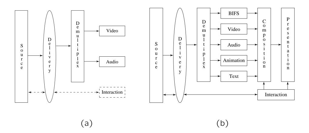
Fig. 12.2: Comparison of interactivities in MPEG standards: (a) reference models in MPEG-1 and 2 (interaction in dashed lines supported only by MPEG-2); (b) MPEG-4 reference model.
