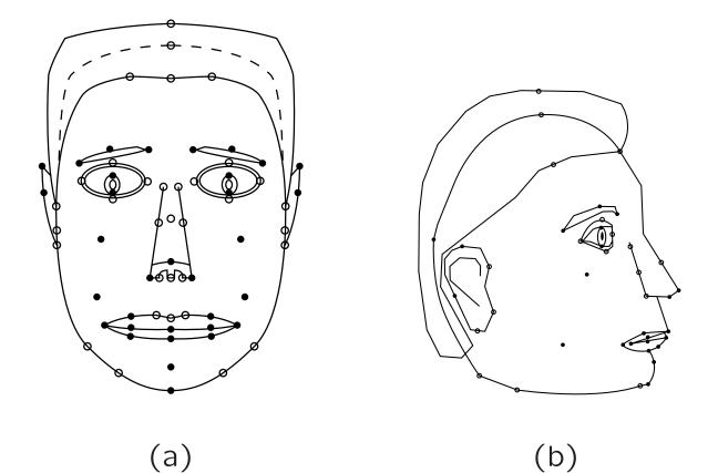
Fig. 12.16: Feature Points for Face Definition Parameters (FDPs). (Feature points for teeth and tongue not shown.)
