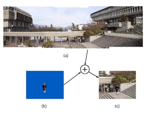
Fig. 12.10: Sprite Coding. (a) The sprite panoramic image of the background, (b) the foreground object (piper) in a blue-screen image, (c) the composed video scene.
