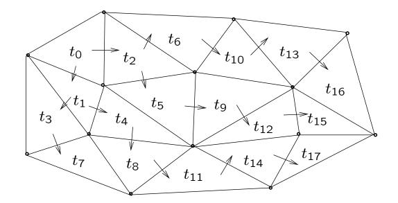
Fig. 12.14: A breadth-first order of MOP triangles for 2D mesh motion coding.
