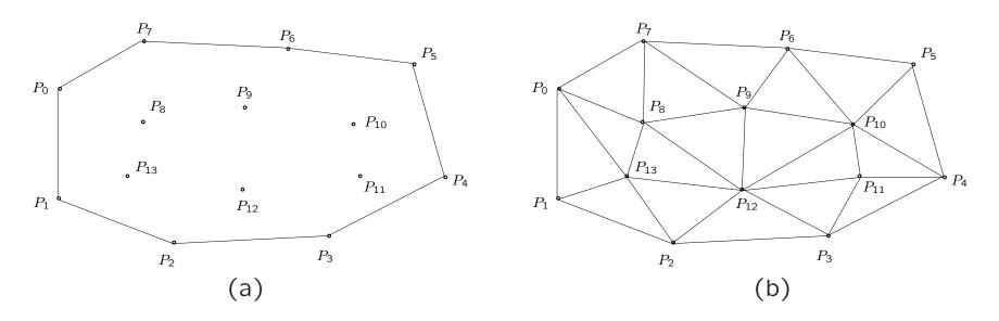
Fig. 12.13: Delaunay Mesh: (a) Boundary nodes ( $P_0$  to  $P_7$ ) and Interior nodes ( $P_8$  to  $P_{13}$ ). (b) Triangular mesh obtained by Constrained Delaunay Triangulation.
