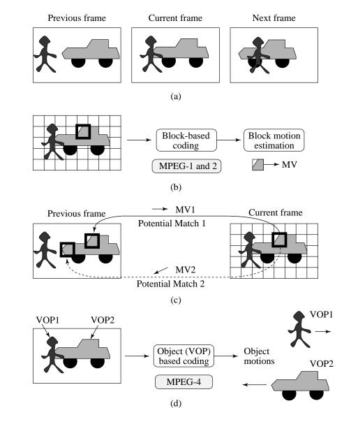
Fig. 12.4: Comparison between Block-based Coding and Object-based Coding.
