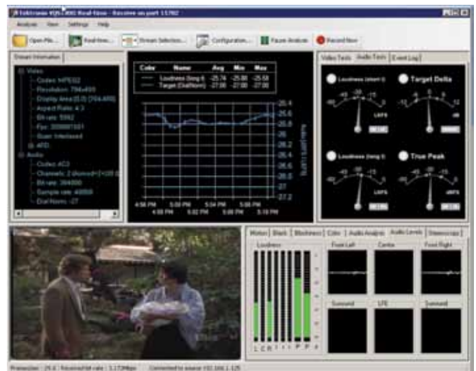
Figure 13-5. Cable broadcast with audio at 2 dB louder than DialNorm. This is a 4 dB increase over the satellite feed.
