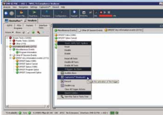
Figure 13-13. MTS4000 Transport Stream Compliance Analyzer enabling the CaptureVu and Recording for SCTE35 DPI packets.
