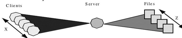
Figure 11. Process-per-Server ( $X+Z$  connections)
