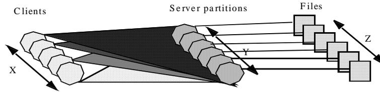
Figure 12. Process-per-Application-per-Server Partition ( $X+1$  connections per server)
