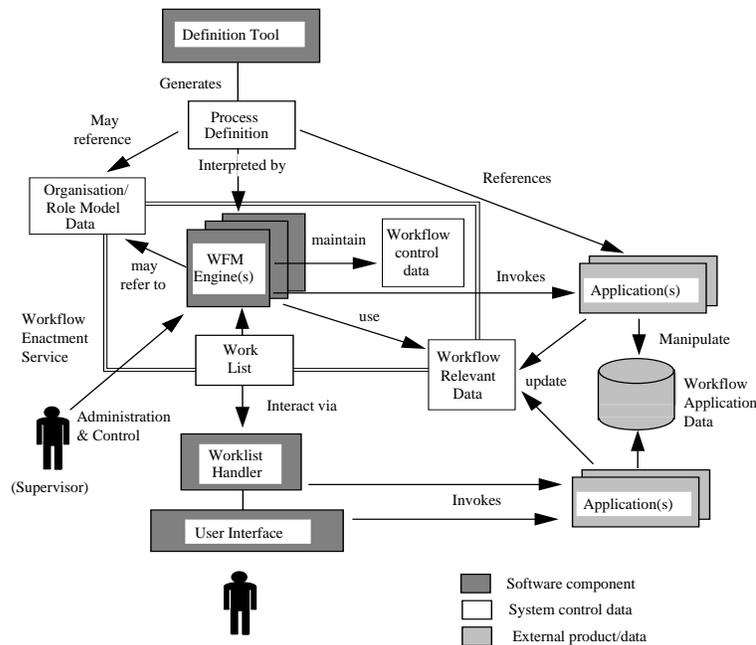
Figure 5. WFMS capabilities and data as defined by the WfMC Reference Model
