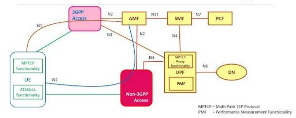
Based on 3GPP TS 23:501 4.2.10-1: Non-roaming and Roaming with Local Breakout architecture for ATSSS support
