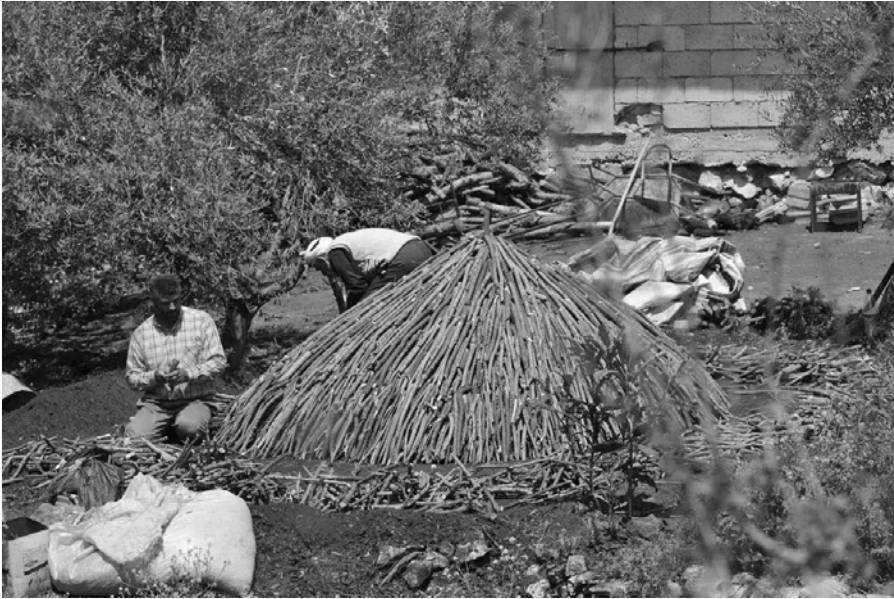
Preparing wood for charcoal near Bzel, Lebanon. Oaks are favored for the production of the highest-quality charcoal.
