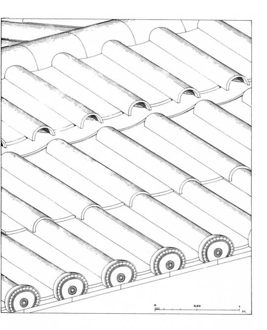
Figure 2. Laconian tiles: roof of the Heraion at Olympia (after Hesperia 59 [1990] 15).
