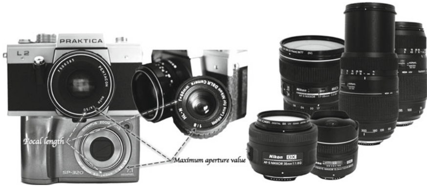
Fig. 4.10 Prime and zoom lenses and their specifications
