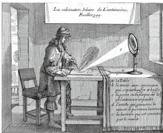
Fig. 2.2 Nicaise le Fèvre's drawing of the calcination of antimony by focused sunlight
