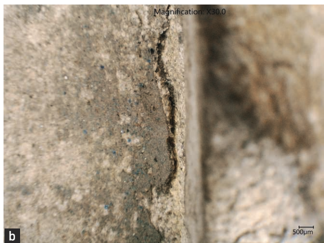
Fig. 6 a-b. a. Picture panel of funerary slab with a soldier taking a kantharos from his attendant (fig. 1 e). © The Metropolitan Museum of Art/B. Schwarz; b. Detail of lead white preparation layer visible below dark background color at right edge of picture panel, approximately 9 cm from the bottom edge of the picture panel, magnification 30x. Image taken in situ on panel using a Keyence digital microscope VHX-6000 with a VH-ZST dual objective low power (20-200x) zoom lens mounted on tripod. © The Metropolitan Museum of Art/D. Abramitis.
