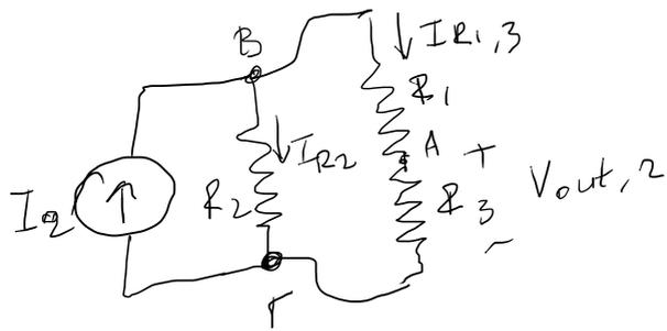
$$V_{B\Gamma} = I_2 \cdot (R_2 \parallel (R_1 + R_3))$$
