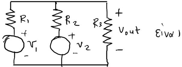
$$V_{out} = V_{out,1} + V_{out,2} \quad \text{όπου}$$
