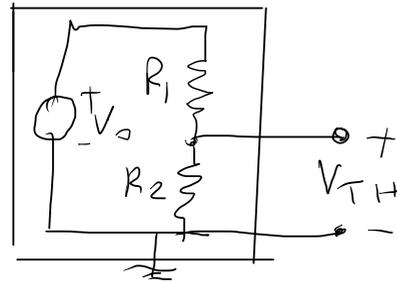
$$V_{TH} = V_0 \cdot \frac{R_2}{R_1 + R_2}$$
