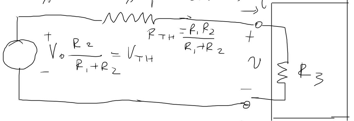
$$V = V_{TH} \cdot \frac{R_3}{R_{TH} + R_3}, \quad i = \frac{V}{R_3} \quad \text{δηλαδή} \quad V = V_0 \cdot \frac{R_2}{R_1 + R_2} \cdot \frac{R_3}{\frac{R_1 R_2}{R_1 + R_2} + R_3} =$$
