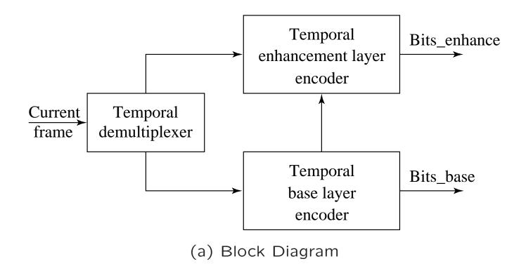
Fig 11.10: Encoder for MPEG-2 Temporal Scalability.
