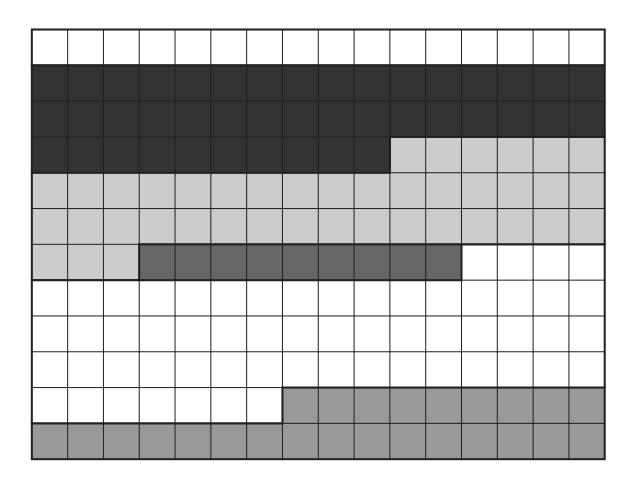
Fig 11.4: Slices in an MPEG-1 Picture.
