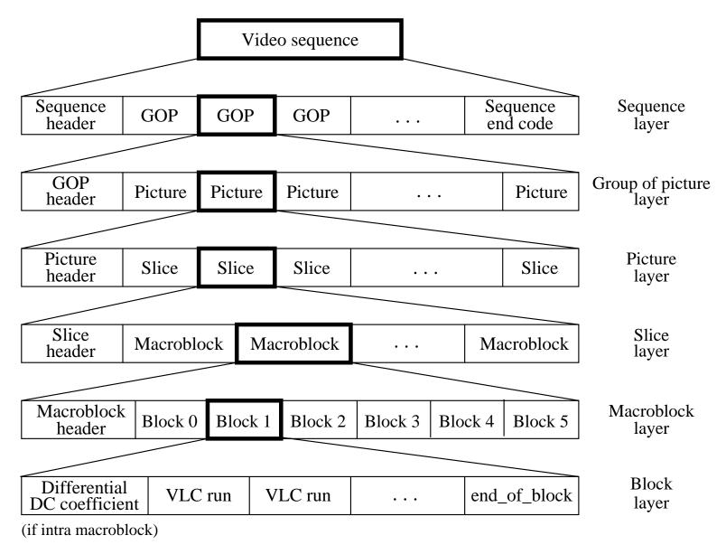
Fig 11.5: Layers of MPEG-1 Video Bitstream.
