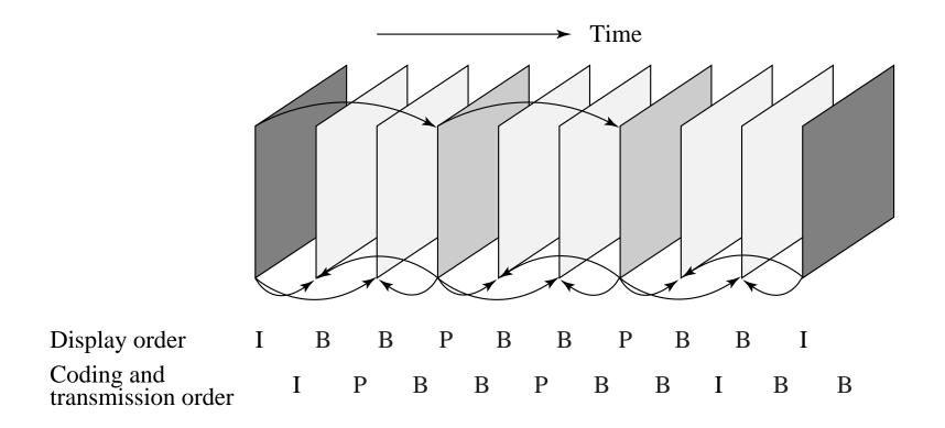
Fig 11.3: MPEG Frame Sequence.
