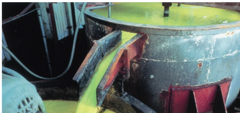
Figure 15.4 Ammonium diuranate (yellowcake) after solvent extraction (Photo from UIC). (See insert for color representation of the figure.)
